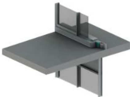
Low performing detail – Traditional Concrete Balcony 16
